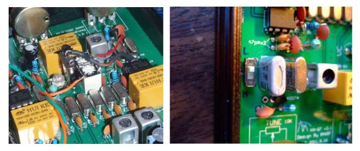
By design, the KN-Q7A has limited tuning capability. In order to add additional band coverage in the 40 Meter band, you need to add an additional crystal.
